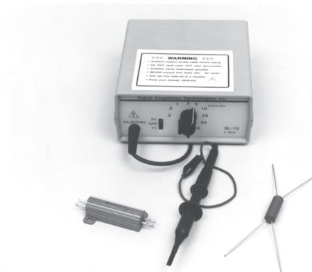
Figure C3. Typical Current Shunts and an "Isolated" Probe
